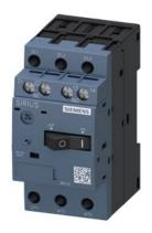
Circuit breaker size S00 for motor protection, CLASS 10 A-release 7...10 A N release 130 A Screw terminal Standard switching capacity with transverse auxiliary switch 1 NO+1 NC
